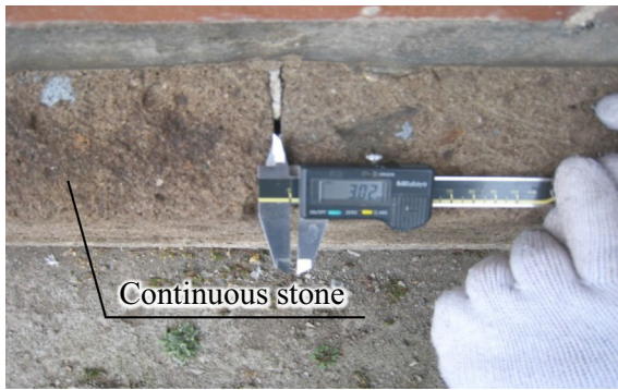
Photograph 4. Gap between continuous stones measured using a vernier caliper.
